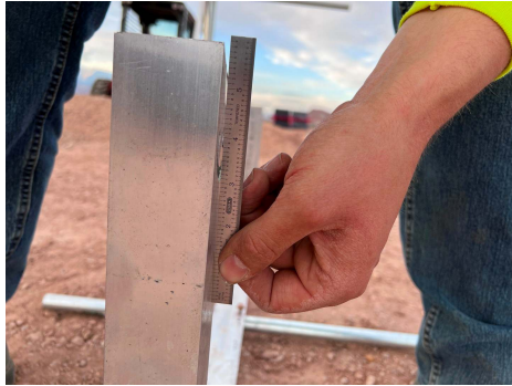
PHOTO 10: Slight deformation after load removed
