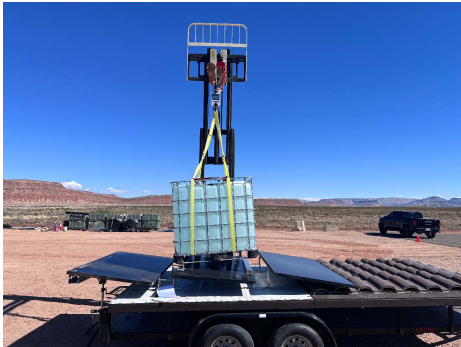
PHOTO 1: Weighing the large water tank
